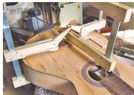
▲ Pic.26 ...and glued into position – Phil used a modified clamp for extra reach in the soundhole
